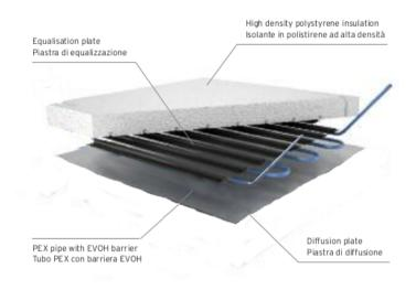
The large surface of heat distributed homogeneous avoids thermal stress to materials increasing the stability of the materials and the duration of the system over time. The insulator, finally, ensures that almost all the heat supplied to the panel goes toward the metal distribution avoiding waste due to unwanted transmissions of heat to areas not of interest.
