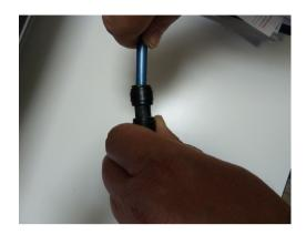
The outlet piping from the panel are compeltate with an anti-occlusion, isolation from a closed cell polyurethane and a junction joint type fast-plug.
